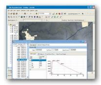
Pipeline spill volume is accurately calculated in a time versus flow rate hydrograph.
